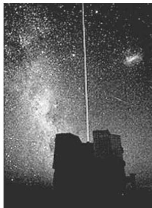
The bright line is a laser beam visible only because of atmospheric scattering.
